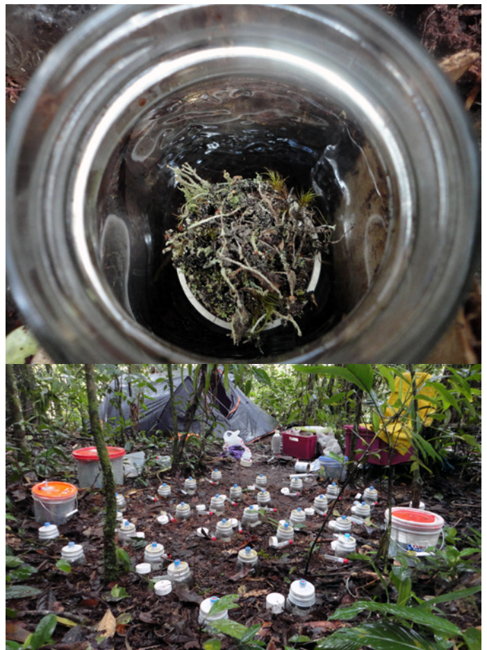
Figure 16: To measure N_2 fixation intact soil cores from the canopy and forest floor were placed in jars ( top ), which were then sealed, and 10% of the headspace air was replaced with acetylene gas. The jars were installed in the forest floor just outside each NUMEX site ( bottom – near the Bombuscaro site) and gas samples were taken from the jars four times during the 24 hours of incubation. Ethylene flux was converted to N_2 fixation using the literature ratio of 3.9:1 as described in [1]. Photos: Amanda Matson
